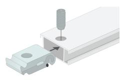
Then put the stabilizer (BFSTS) on the lockset, now tighten the screw with the delivered allen key.
