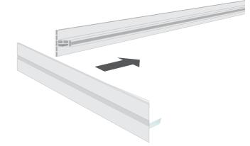
When connecting the frame, first place the lockset (BH0200) without the punchholes, then the one with punchholes.
