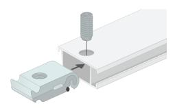
Then put the stabilizer (BFSTS) on the lockset, now tighten the screw with the delivered allen key.
