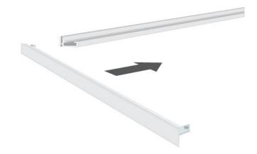
When connecting the frame, first place the lockset (BH0210) without the punchholes, then the one with punchholes.
