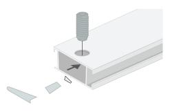
Then put the stabilizer (BFSTS) on the lockset, now tighten the screw with the delivered allen key.
