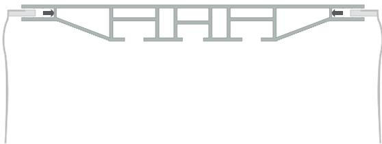
Place the textile print in the frame. Start with the corners and press the silicone strip in the channel.
