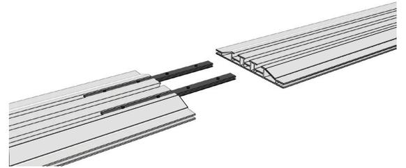
These extension sets can be placed in the channels where the frame is cut in half.
