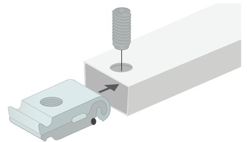
Put the stabilizer on the lockset, now tighten the screw with the delivered allen key.
