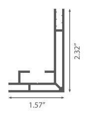
Single-sided fabric frame, suitable for wall mounting. The frame is only 2.32" thick, it has an elegant look and is suitable for many solutions. This aluminum profile is designed to give an exquisite illumination to your textileprint.
