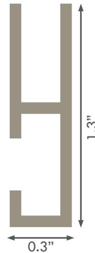
Single-sided textile frame, meant to be built in. This profile is often mounted in a niche. Due to its simplicity, it is an ideal solution for a low cost textile frame.
